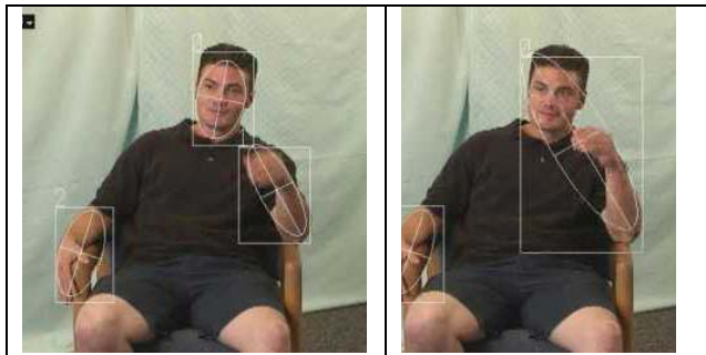
Figure 6. Hand and head blobs merging
