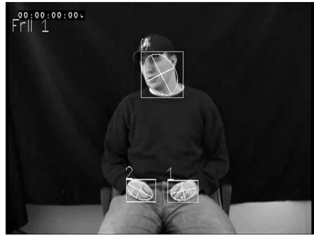
Figure 1. Blobs capture the location of the head and hand
